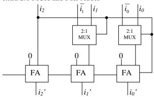
The Full Adder is implemented as shown below. Half Adders could also be used, but for the sake of minimizing different functional pieces in the design, I've chosen to use only Full Adders.
