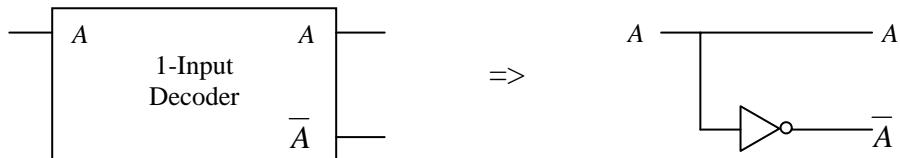
Therefore, using this and some AND gates, we can decode the signals as follows:
