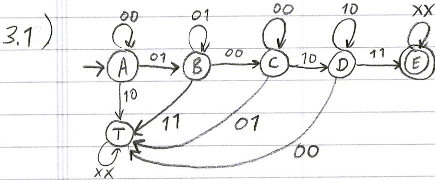
Four adj. to T. Need 4 state variables before state splitting. However, using multiple T states permits 3 variables.
