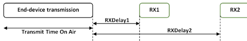
Fig. 2. Bidirectional communication between end-device and base station for LoRaWAN class A.
