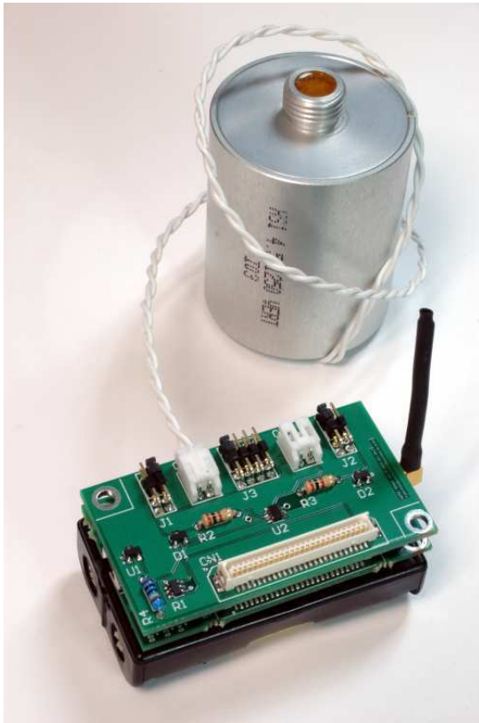
Figure 1: Geophone connected to Shake 'n Wake board mated to Crossbow mote.
