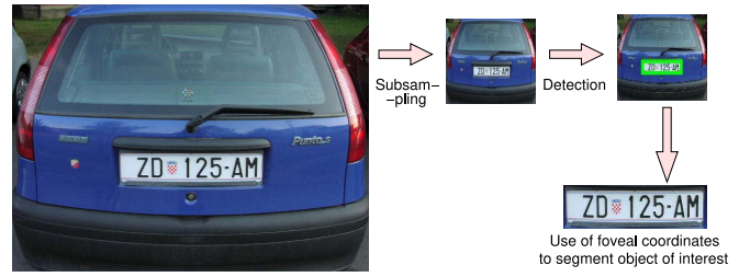
Fig. 7. Demonstration of digital foveation in license plate recognition. A high-resolution image is subsampled and used to identify the region of interest, which is used in high-resolution capture and analysis.
